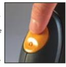
**Note.** It takes a few operations to get used to switching the sander on and off due to the protective cover. However, it is well worth the effort due to the protection afforded to the switch and the consequent increased lifetime of the unit.
